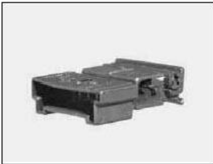
Fig. 147: Identifying 6-Pin MQS Plug
