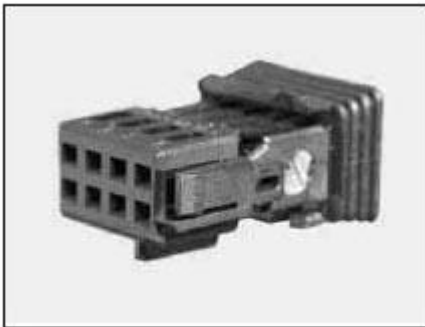
Fig. 113: Identifying 8-Pin MOS Coupling
