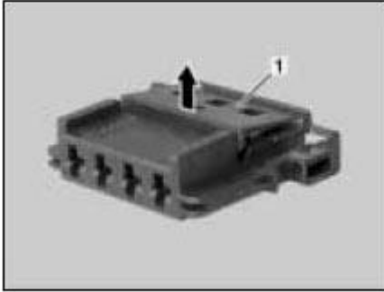
Fig. 525: Lifting Locking Shackles - Shown On A 4-Pin MCP Coupling
