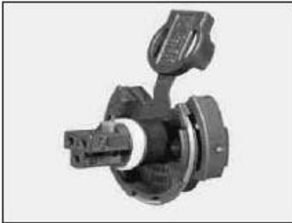
Fig. 123: Identifying 3-Pin MQS Coupling
