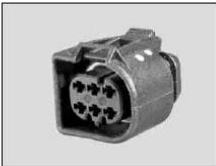
Fig. 96: Identifying 2X3-Pin SLK Coupling
