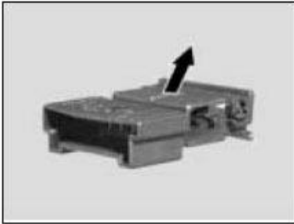
Fig. 442: Opening Contact Retainer - Shown On 6-Pin MQS Connector
