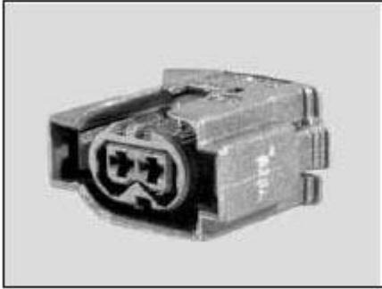
Fig. 87: Identifying 2-Pin SLK Coupling
