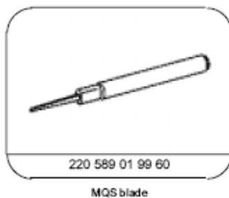
Fig. 457: Identifying MQS Blade (220 589 01 99 60)
