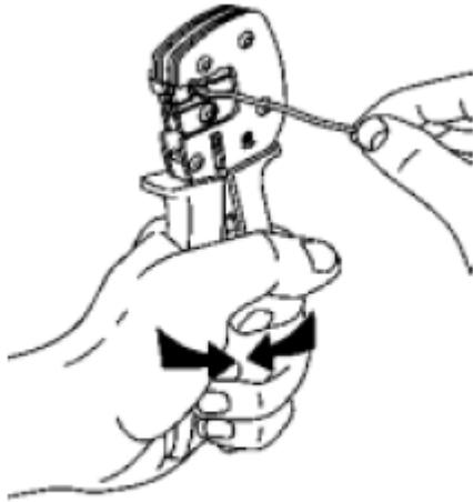
Fig. 378: Squeezing Crimp Pliers
