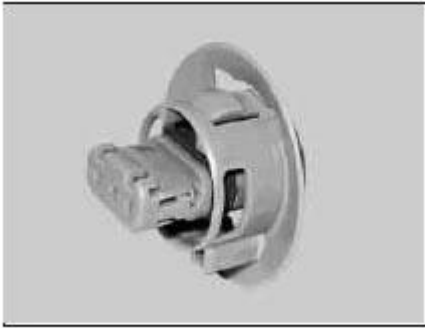
Fig. 181: Identifying 3-Pin MQS Coupling
