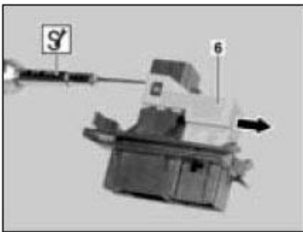
Fig. 516: Prying Up Lock Tab On Retaining Cap - Shown On 4/8-Pin JPT/MQS Plug
