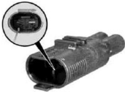
Fig. 261: Identifying 2-Pin LSK, Plug
