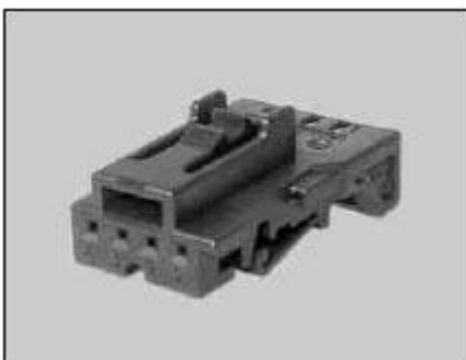
Fig. 179: Identifying 14-Pin, MOS Coupling
