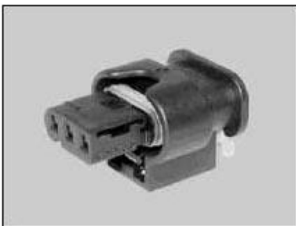
Fig. 306: Identifying 3-Pin MLK Coupling
