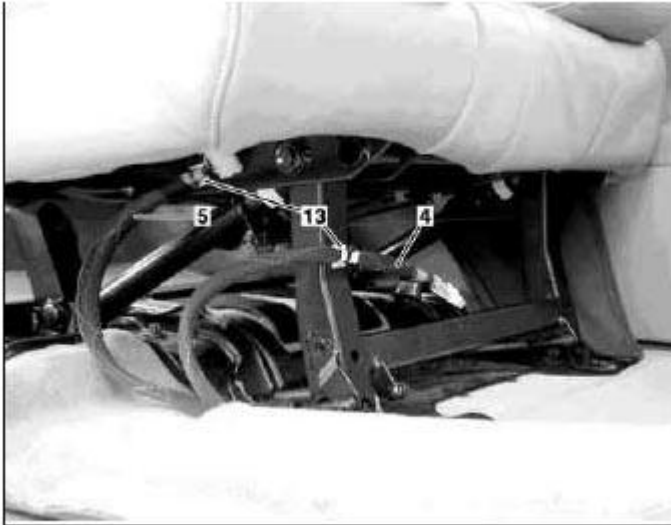
Fig. 253: Identifying 4-Pin SPT Coupling
