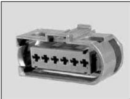
Fig. 88: Identifying 6-Pin SLK Coupling
