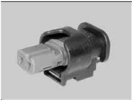
Fig. 305: Identifying 2-Pin MLK Coupling
