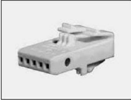
Fig. 128: Identifying 5-Pin MQS Coupling
