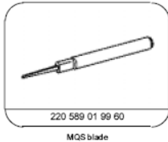
Fig. 470: Identifying MQS Blade (220 589 01 99 60)
