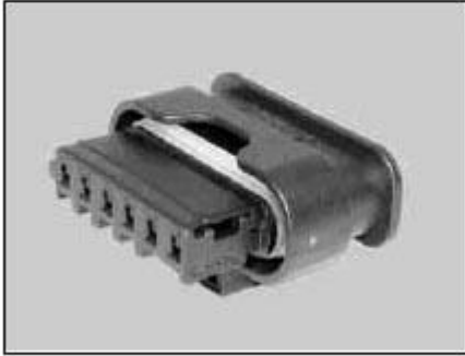
Fig. 310: Identifying 6-Pin MLK Coupling
