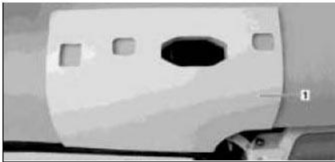
Fig. 568: Opening Lock Tab - Shown On A 2-Pin RK 2.5 Coupling
