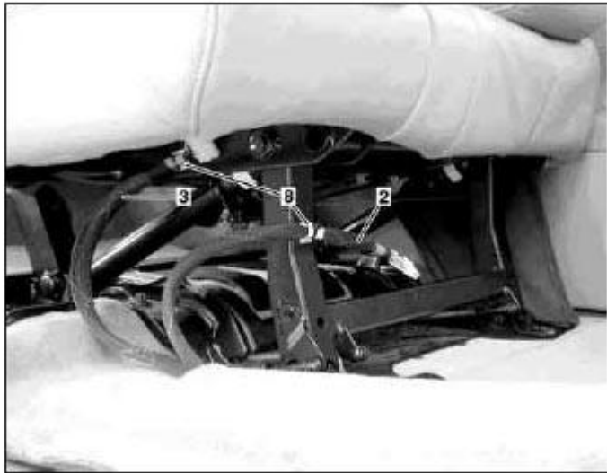
Fig. 258: Identifying 7-Pin SPT Coupling
